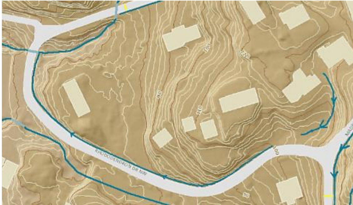
Figure 60. Rhododendron Drive overview and the direction of the water flow.
