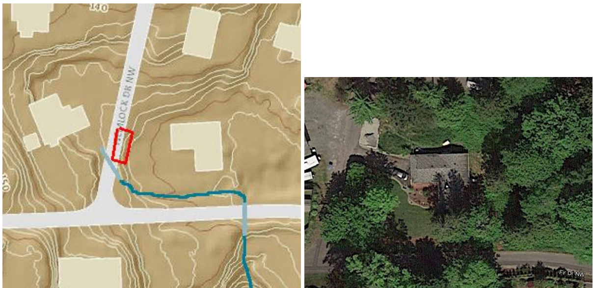
Figure 2.3-2.4, contour map showing drainage route through 242 Hemlock Drive and overview. Red box area denotes driveway entrance onto Hemlock Drive.
