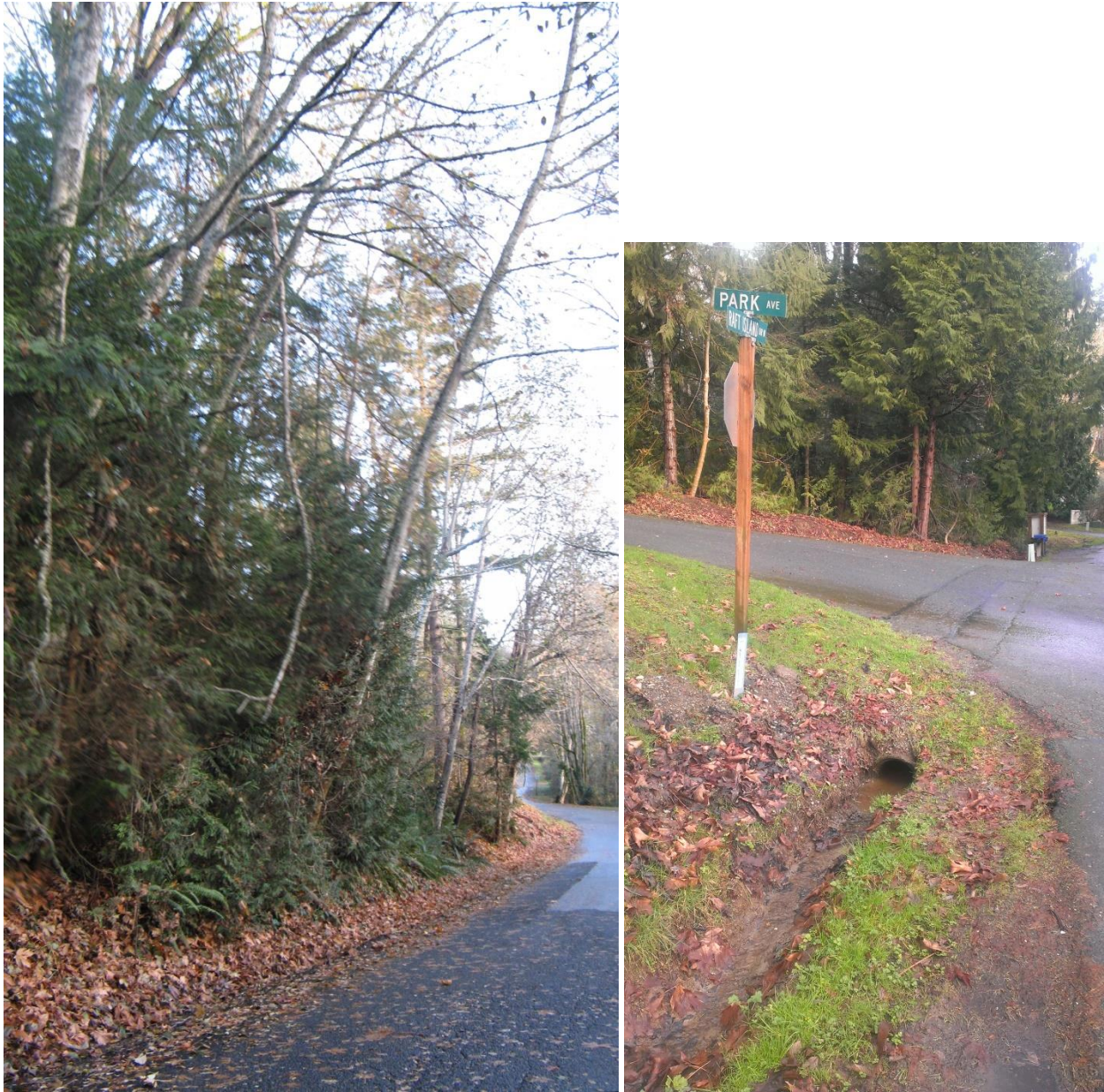
Figure 36. Shoulder on east side of Raft Island Drive and catch basic needed at Park and Raft Island Drive (Plot 4995100480).
